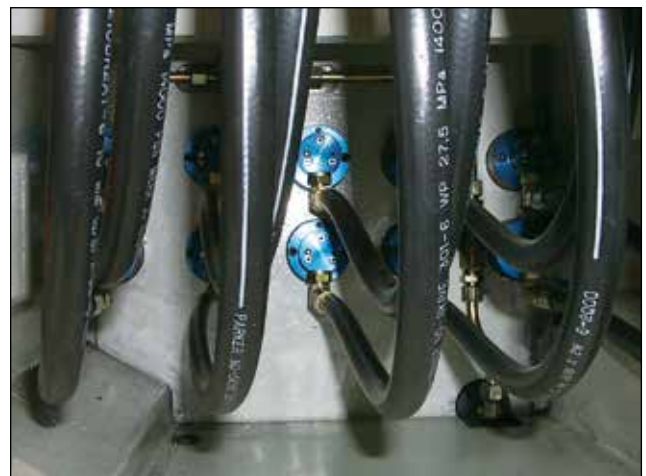
DEUBLIN 1117 Bearingless Unions on Automotive Transfer Line
