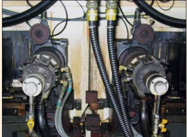
DEUBLIN 2-passage Unions on CNC Turning Center
