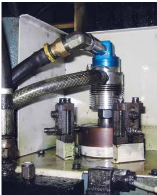
DEUBLIN 1109 on vertical machining center
